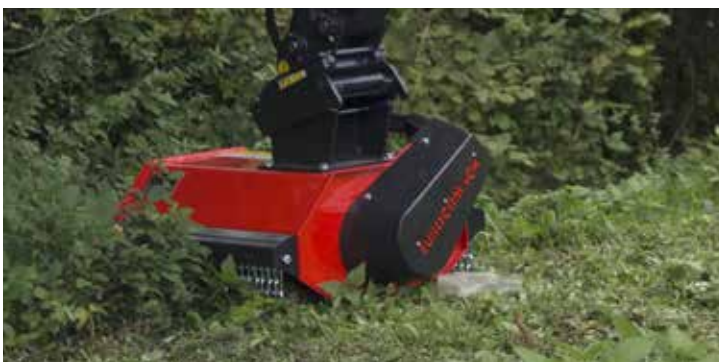
Hydraulic system for cutting head with additional pump (20 l/min)
